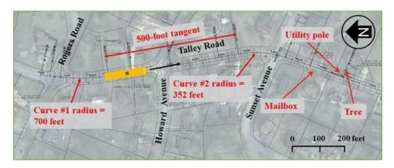
**Figure C-4.** Horizontal curves immediately preceding Talley Road crash location (Source: city of Chattanooga, modified)
